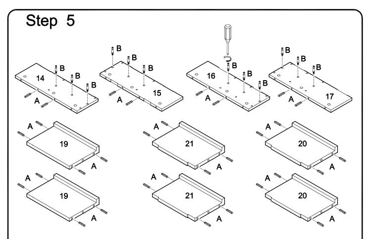
Screw cam bolts (B) and insert dowels (A) into panels (14,15,16,17). Insert dowels (A) into shelves (19,20,21).
